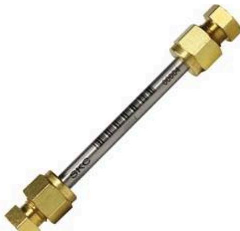
Photo 3: An example of the VOC Passive Diffusion Tube used in the study.
