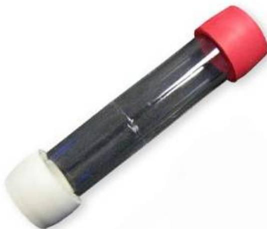
Photo 4: An example of the Passive Diffusion Tube used to monitor  $\text{SO}_2$ ,  $\text{O}_3$  and  $\text{NO}_2$  in the study.
