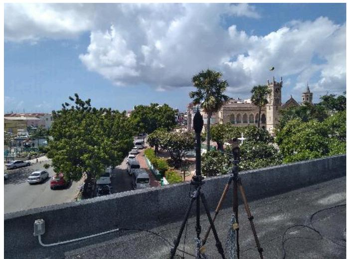
Photo 1: Noise monitoring station set up on the roof of the Treasury Building in Bridgetown
